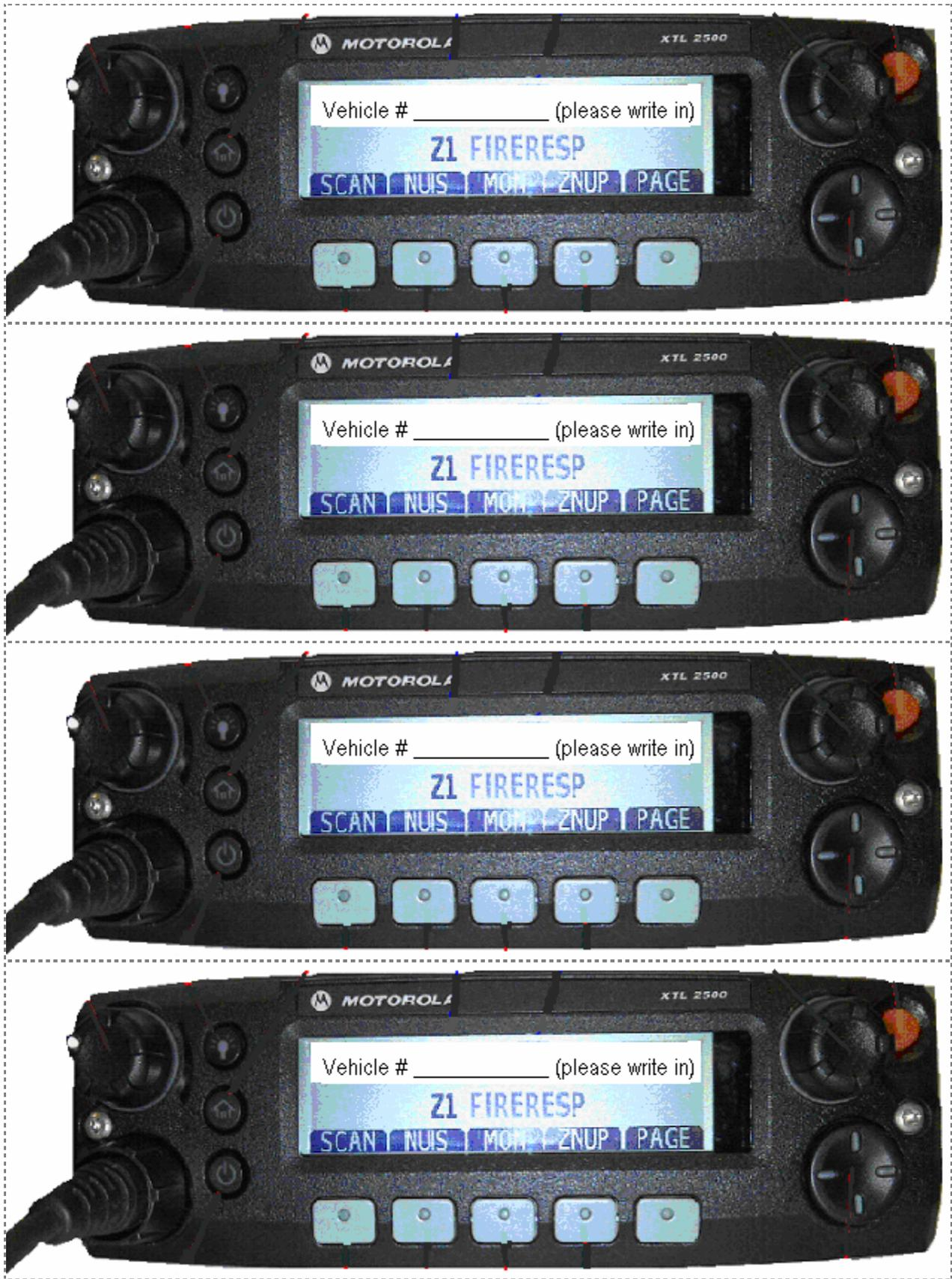
Cut-outs for mobile radio heads – tape to where it is to be mounted in vehicle
